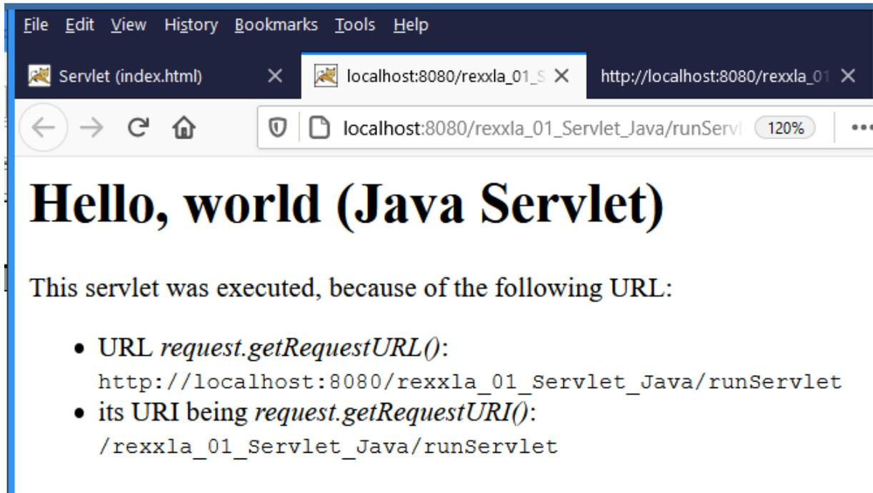
Figure 3: Response to client which was created by the Java servlet.
