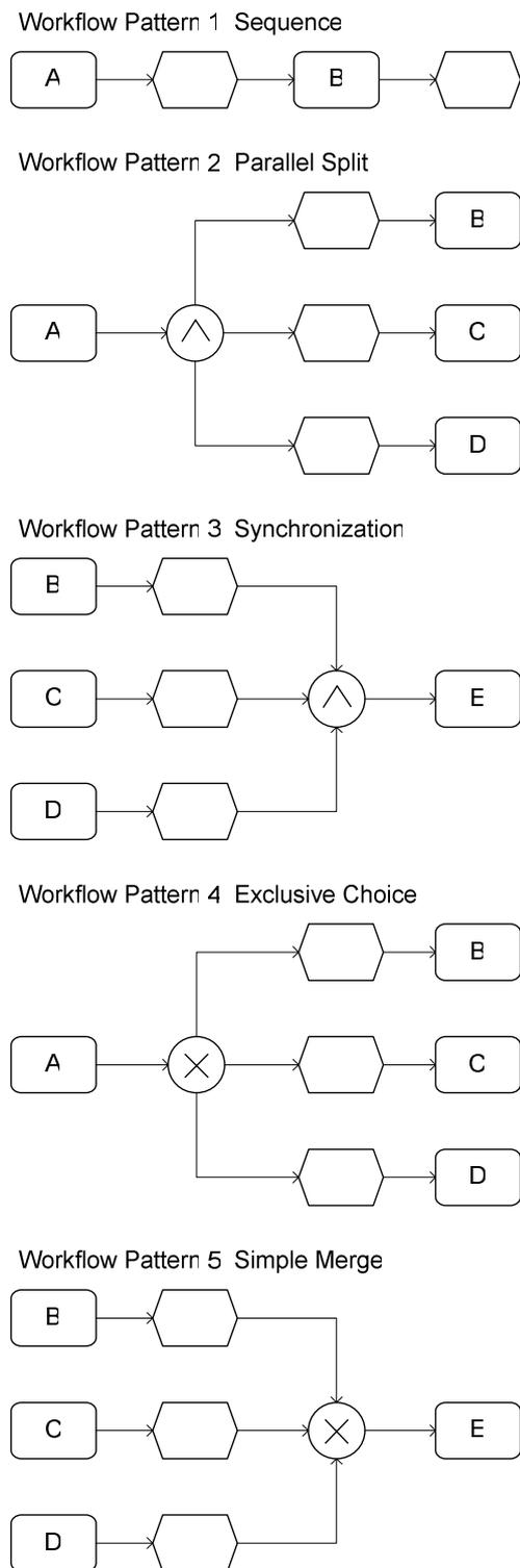
Figure 2: Workflow Patterns 1-5 as EPC models
