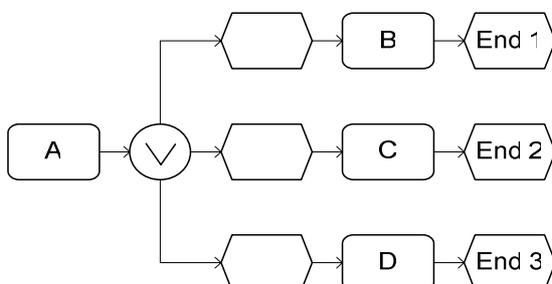
Figure 3: Workflow Patterns 6, 7, 10, and 11 as EPC models
