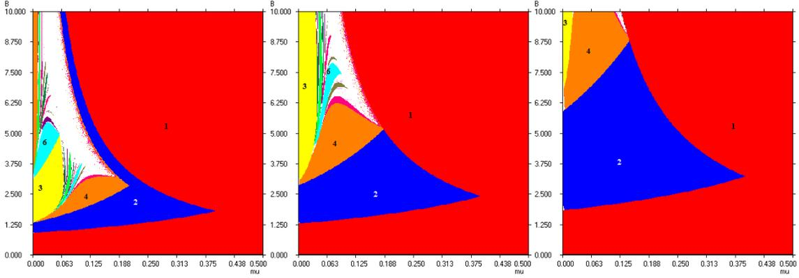
**Fig. 3:**  $(\mu, B)$  plane with  $\gamma = 0.05$  (left),  $\gamma = 0.10$  (center) and  $\gamma = 0.15$  (right). Numbers indicate the periodicity of stable cycles. The white regions indicate a periodicity higher than 12.
