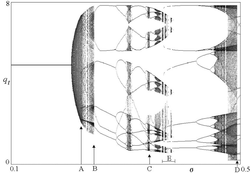
Fig.5 One-dimensional bifurcation diagram of  $q_t$  as a function of  $\sigma$  at  $\delta = 0.9$ . The points A, B, C, D correspond to  $\sigma = 0.22$ ,  $\sigma = 0.245$ ,  $\sigma = 0.34193$ ,  $\sigma = 0.4946$ , respectively. The interval E is enlarged in Fig.7a.
