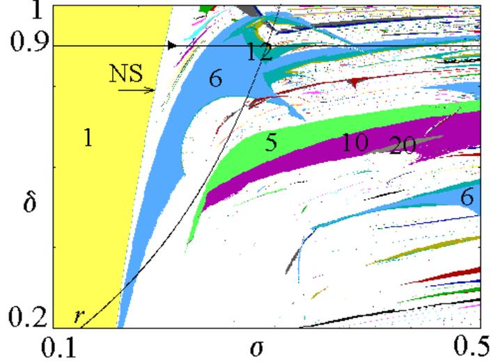
Fig.4 Two-dimensional parameter plane  $(\sigma, \delta)$  at fixed  $a = 8, \nu = 1, m = 2, i = 0.1, \mu = 0.3$ . The different colors denotes regions associated with cycles of different periods. The curve denoted NS represents the Neimark-Sacker bifurcation of the fixed point.
