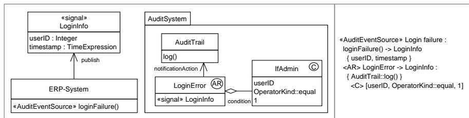
Figure 2: Exemplary graphical and textual concrete syntax [16].
