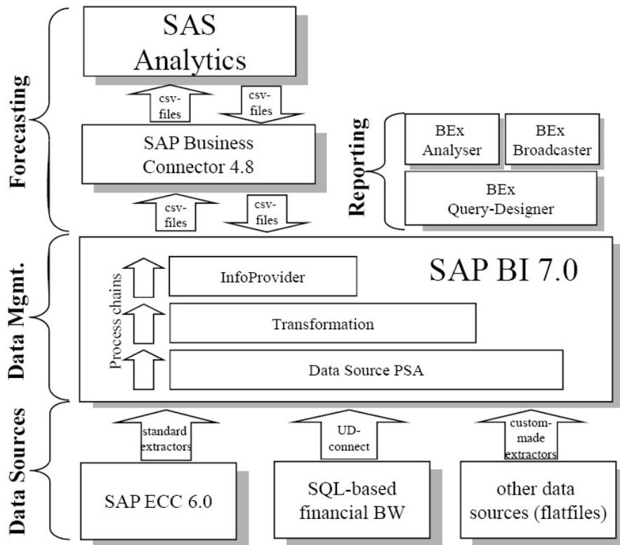
Figure 7: Applied architecture of the planning system.
